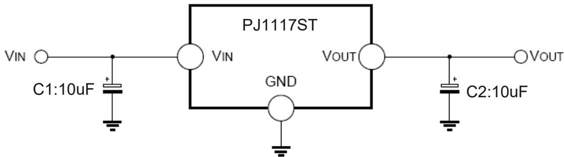
1. Recommend using 10uF tan capacitor as bypass capacitor (C1) for all application circuit.
