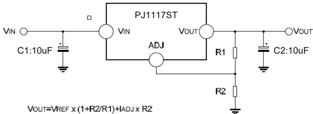
The output voltage of adjustable version follows the equation:  $V_{OUT} = 1.25 \times (1 + R2/R1) + I_{Adj} \times R2$ . We can ignore  $I_{Adj}$  because  $I_{Adj}$  (about 50uA) is much less than the current of  $R1$  (about 2~10mA).
