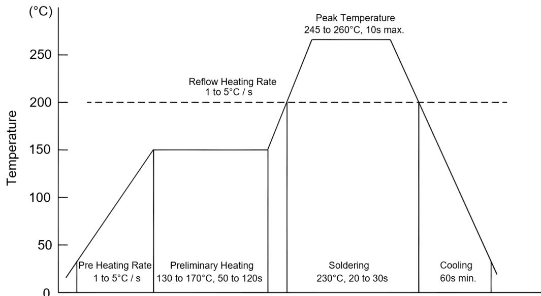
Recommended peak temperature is over 245 °C. If peak temperature is below 245 °C, you may adjust the following parameters:
